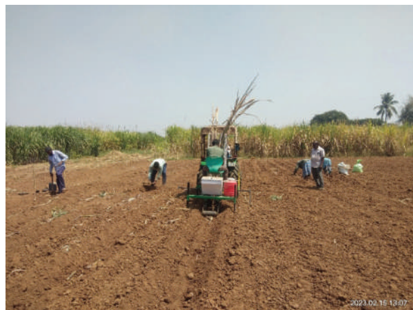
Working of mini tractor-operated sugarcane sett cutter planter in the field
