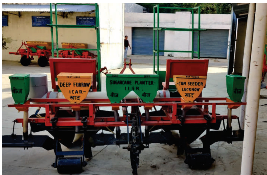
Fabricated Sugarcane sett cutter planter- cum- raised bed multi crop seeder
