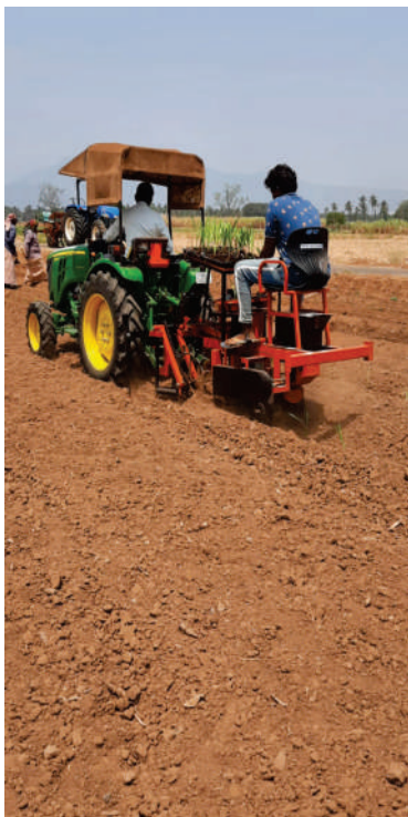
Working of mini tractor-operated sugarcane settling transplanter
