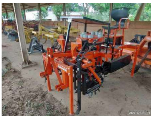
Field testing of tractor-operated whole cane harvester
