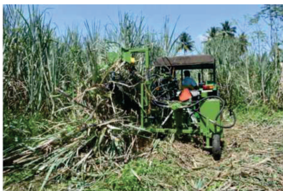
Field testing of tractor-operated whole cane harvester
