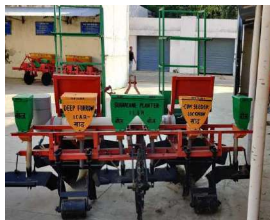
Fabricated Sugarcane sett cutter planter- cum- raised bed multi crop seeder
