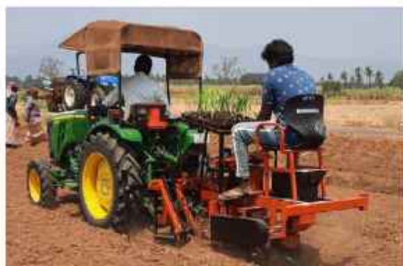
Fig. 37. Mini tractor-operated sugarcane settling transplanter and field view
