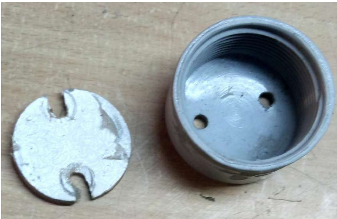
Homemade washer for sensor probes fitting
