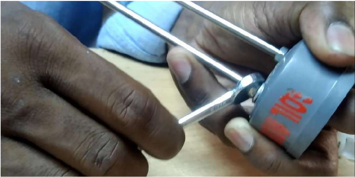
Connector wire to be fitted on the rod with additional washer and nut
