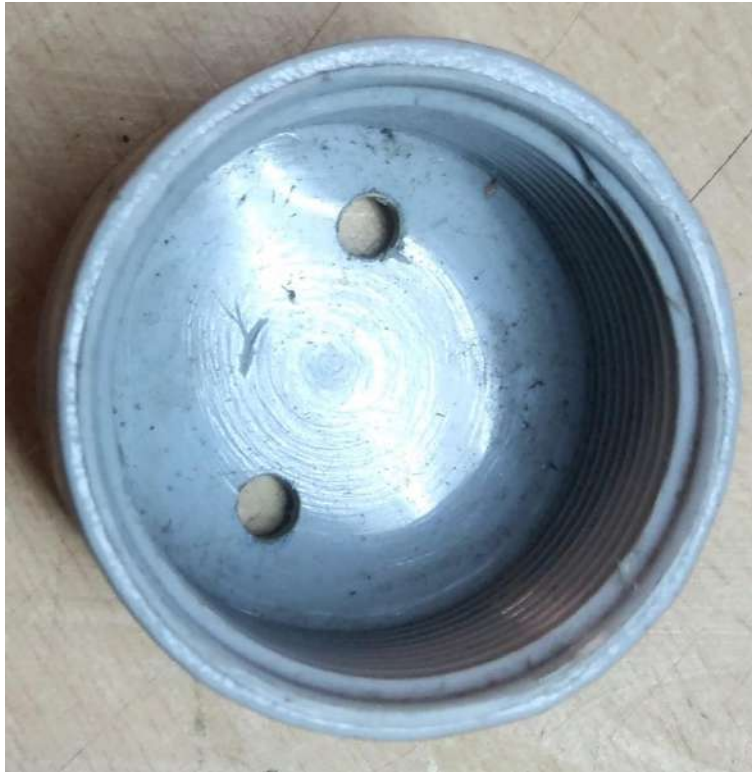
Homemade washer for sensor probes fitting
