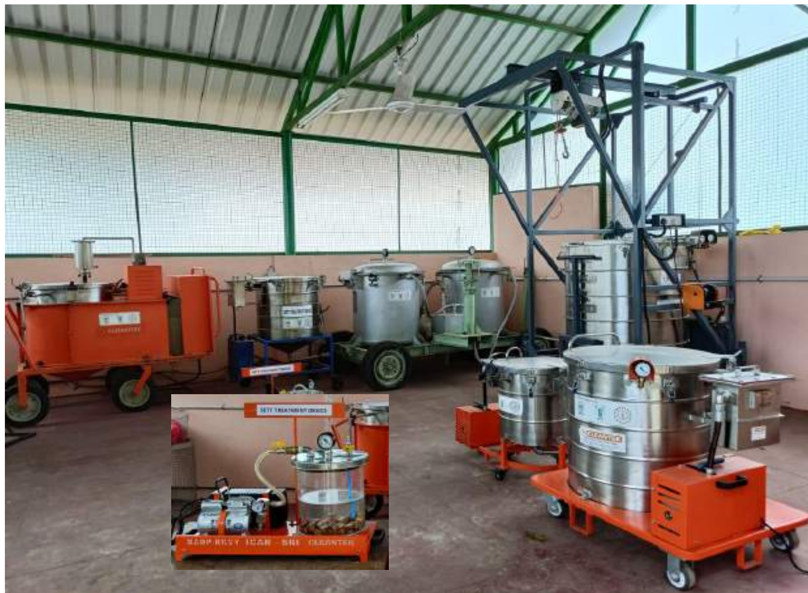
Sett Treatment Chamber at ICAR-SBI
