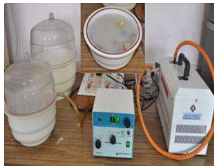
Prototype working under the principle of vacuum infiltration
